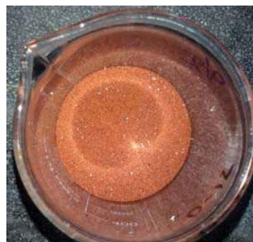
Fig. 1 Iron-oxide coated sand
